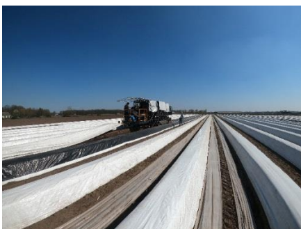
Prototype of Sparter, the 1-row asparagus harvesting robot from Cerescon
