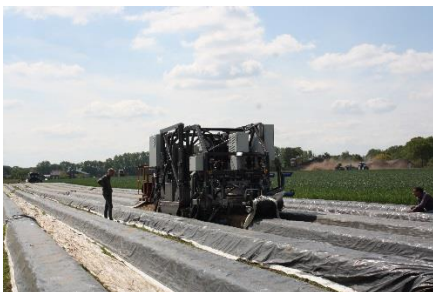
Prototype of Sparter, the 1-row asparagus harvesting robot from Cerescon, in demonstration
