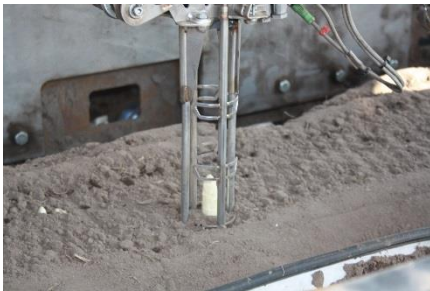
Detail photo 2: asparagus cutting knife from Sparter, the harvesting robot from Cerescon
