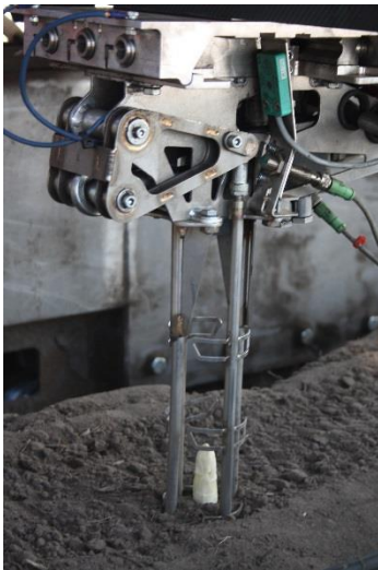
Detail photo 1: asparagus cutting knife from Sparter, the harvesting robot from Cerescon
